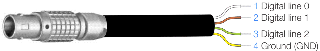
Figure 20: LEMO FGG 00 304 connector with wire colours and description
